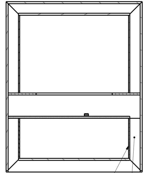
This panel should be removable, to help with fishing mains lead from product to the ground
